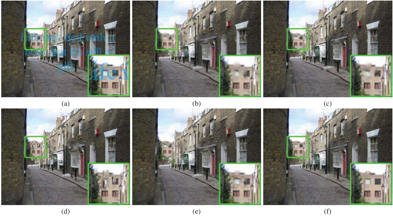
Figure 8. (a) A corrupted image. This image shows more complicated structures. Results obtained by (b) Poisson Image Editing [10] with zero gradient assignment, (c) image inpainting [2], (d) exemplar based inpainting [4], (e) sparse representation [9] and (f) our proposed method.
